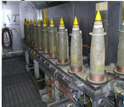
Breaching and Recovery of Bulk Energetics
